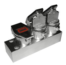
The Type T interlock is an assembly of two or more lock cylinders in a single housing. Type T interlocks are designed to retain one or more keys (called held keys) while the remaining (initiating) key(s) are removed. This allows an exchange of keys in an interlock sequence. All initiating keys must be inserted into the Type T interlock before the held keys can be removed. Once a held key is removed, the initiating keys are trapped in the interlock.
